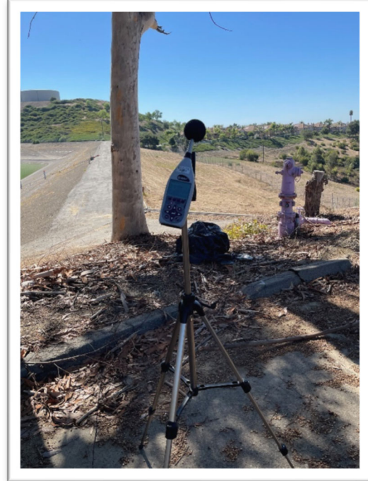
Photograph 4: Ambient and existing plant noise monitoring location looking south. Residential receivers along Hillrise can be seen to the upper right.
