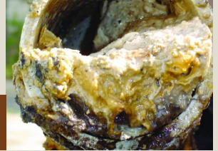
A fatberg caused by fats, oils and grease (FOG)
