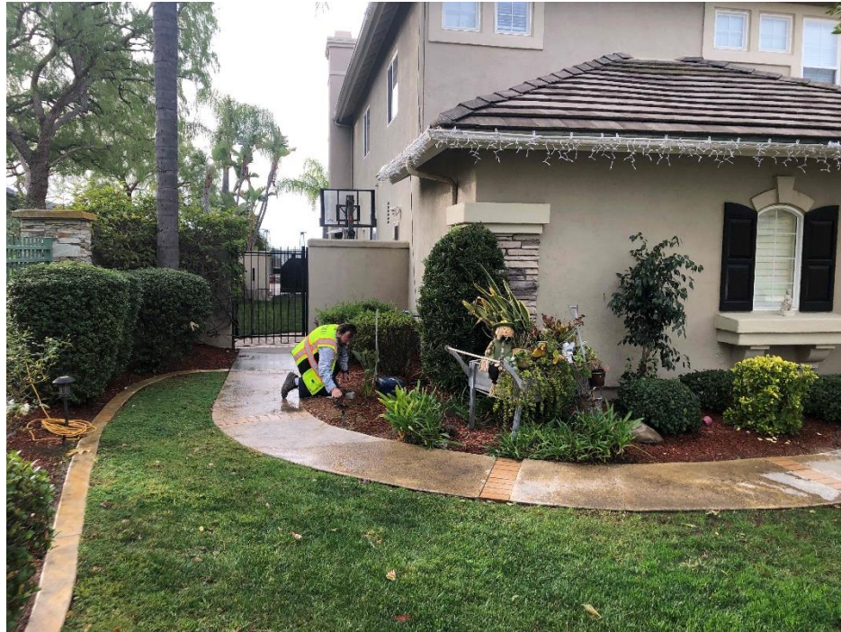
GMU Placing Vibration Monitoring at 95 Bell Canyon
